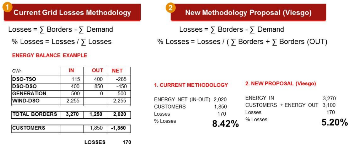
Figure 14: Viesgo's proposal for a new formula for the incentive for losses reduction
